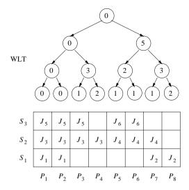
Fig. 2. The binary workload tree (WLT) for the buddy based allocation system.
