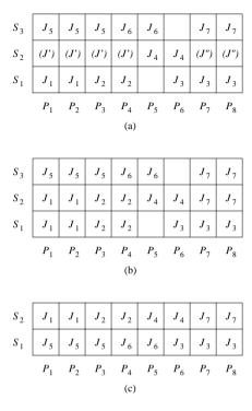
**Fig. 1.** An example of alleviating the fragmentation problem by (b) running jobs in multiple time slots and (c) re-packing job to reduce the total number of time slot.
