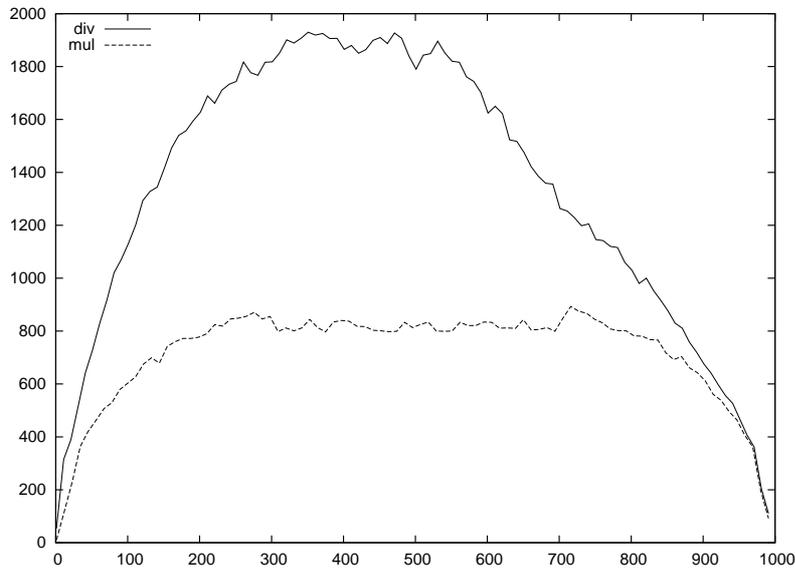
Figure 1.4 Time in  $10^{-5}$  seconds for the multiplication (lower curve) of  $x$  words by  $1000 - x$  words and for the division (upper curve) of 1000 words by  $x$  words, with GMP 5.0.0 on a Core 2 running at 2.83GHz.
