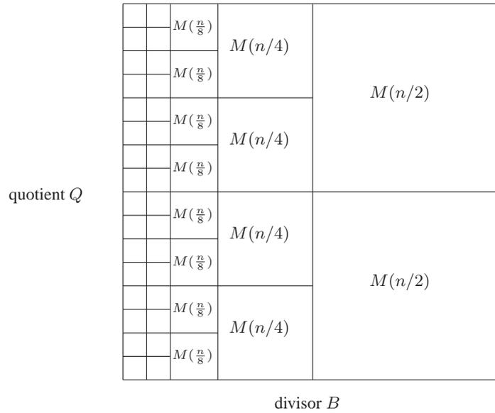
Figure 1.3 Divide and conquer division: a graphical view (most significant parts at the lower left corner).
