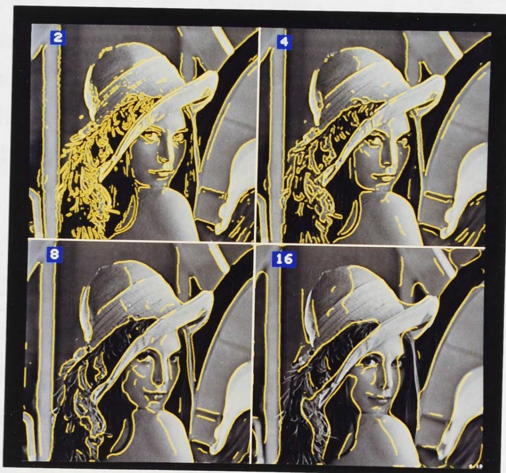
Figure 4.19: Results from Canny edge detector for image lenna
