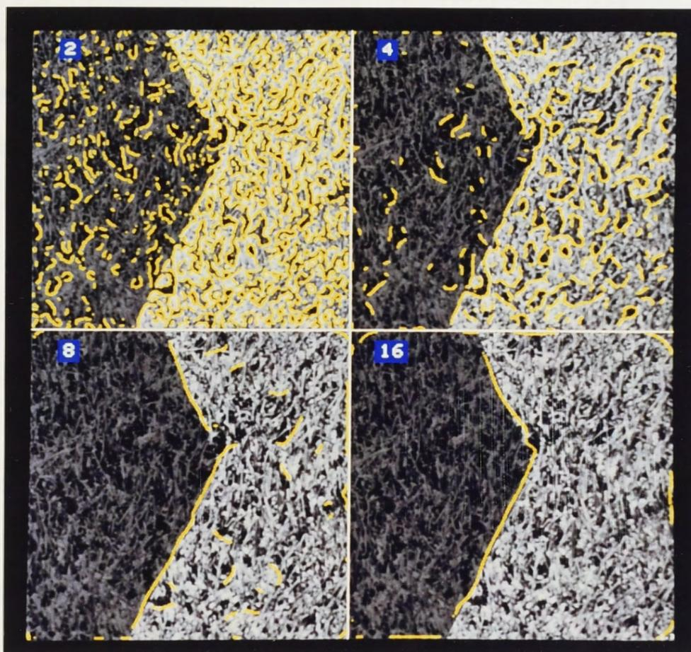
Figure 2.3: Results from figure 2.1 with Canny edge detector
