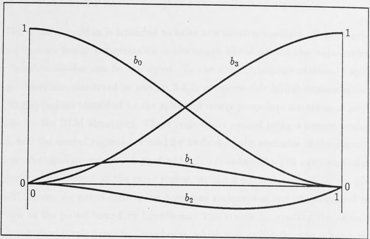
Figure 3.8: Blending functions for cubic segments
