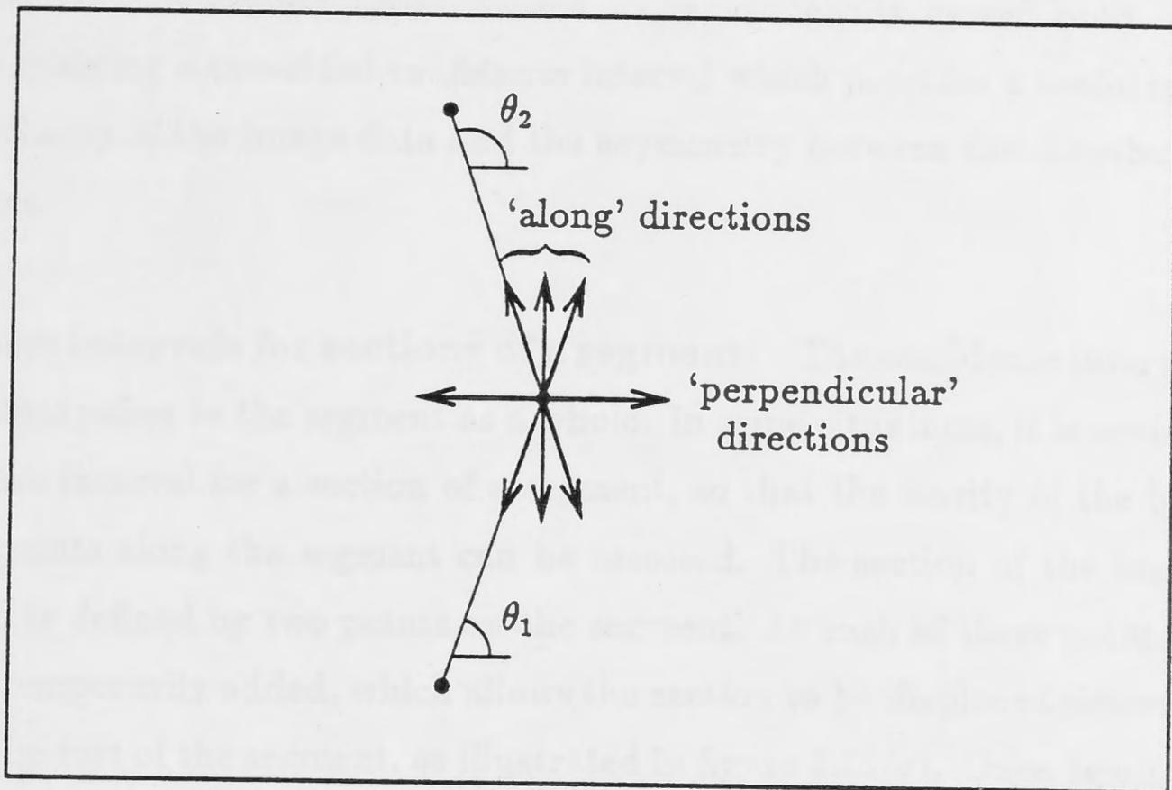
Figure 3.12: Directions used in determining corneriness measure
