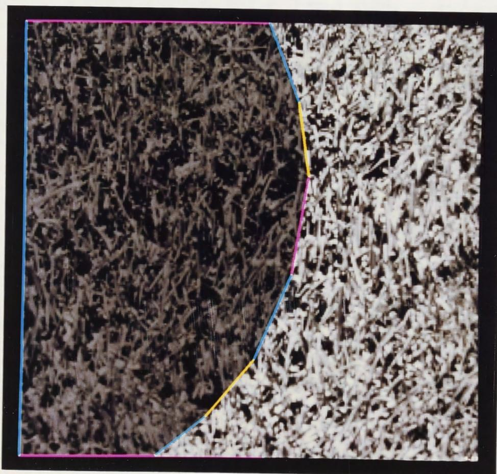
Figure 4.23: Results from BLM algorithm for image gmarc; piece-wise linear boundary
