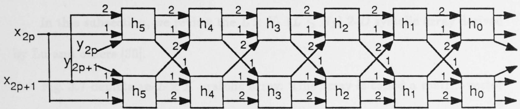
**Fig. 3.6.** 2-D systolic array for a linear phase filter
