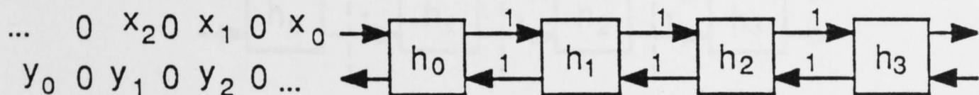
Fig. 2.3. Systolic array for linear convolution in [27]
