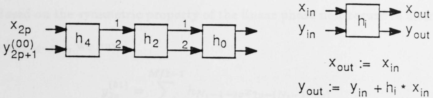
**Fig. 3.1.** Linear systolic array for computing  $y_{2p}^{(00)}$  ( $N_1 = 6$ )
