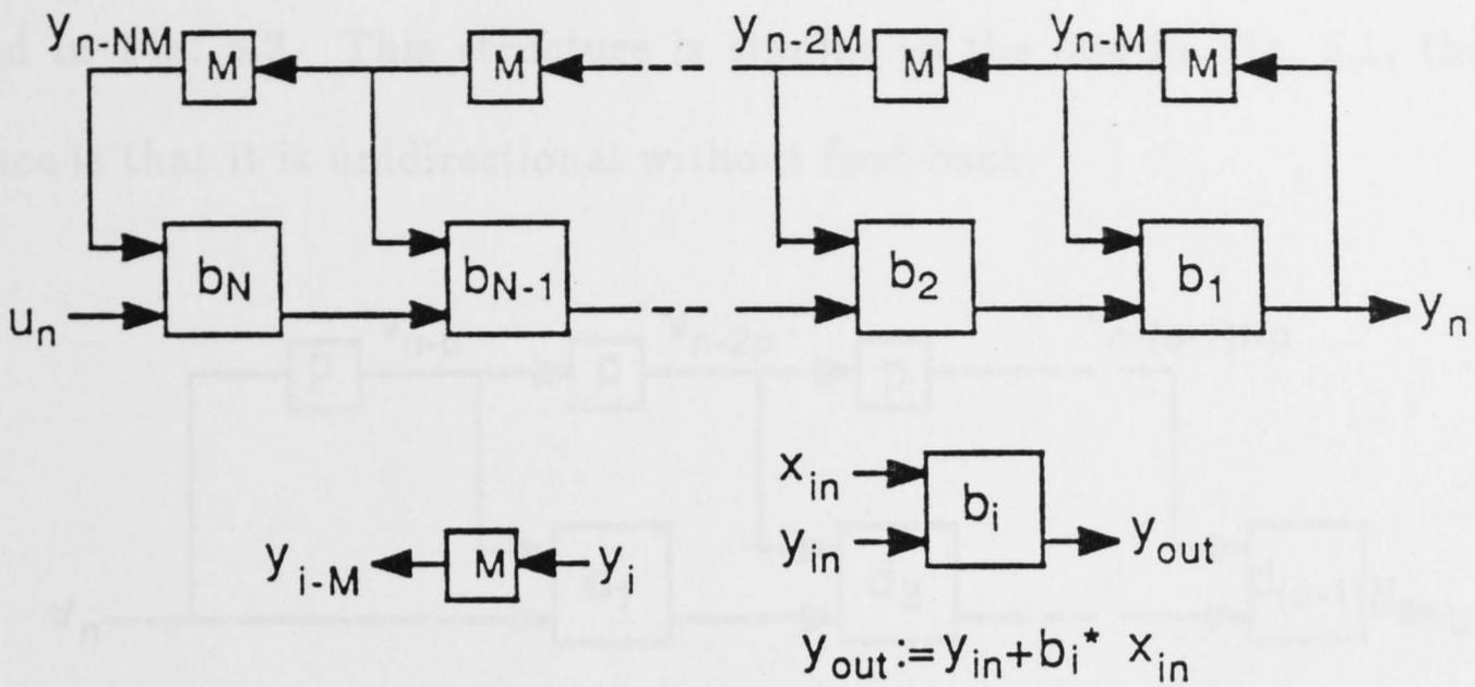
Fig. 5.1. The structure for the recursive part ( $N = 2$  and  $M = 4$ )
