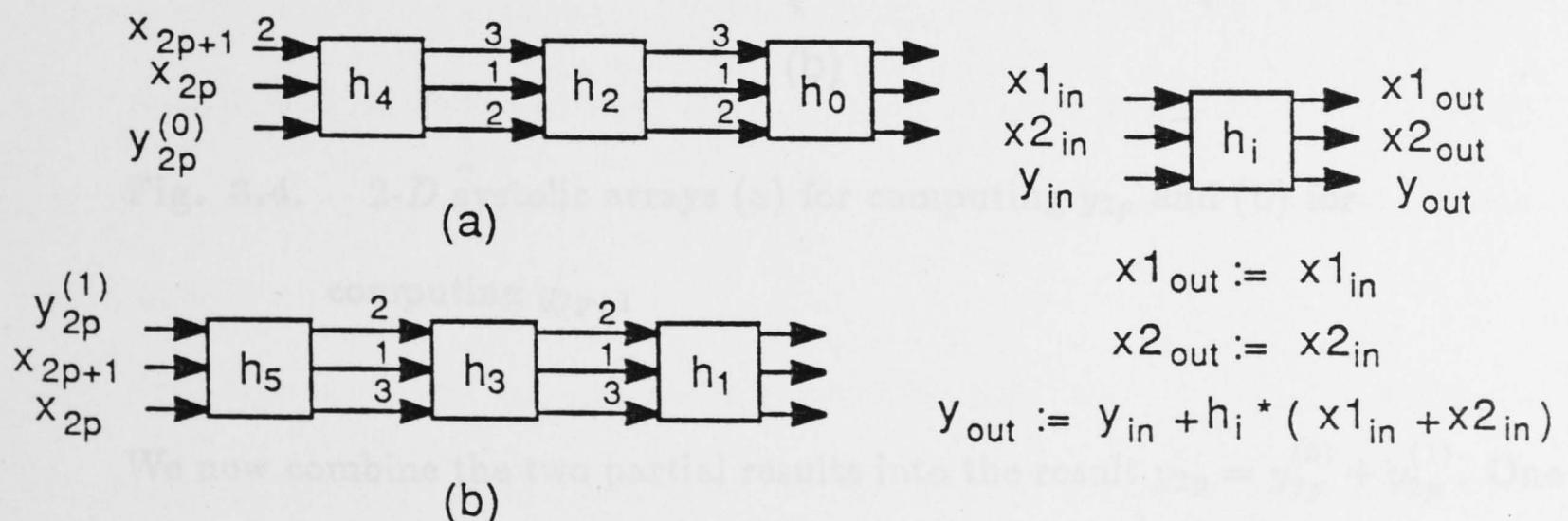
Fig. 3.3. Systolic arrays (a) for computing  $y_{2p}^{(0)}$  and (b) for  $y_{2p}^{(1)}$
