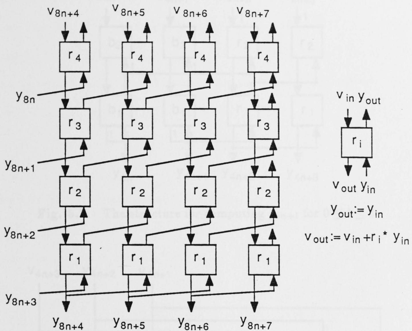
**Fig. 5.6.** The structure for computing  $y_{8n+l}$  for  $4 \leq l \leq 7$
