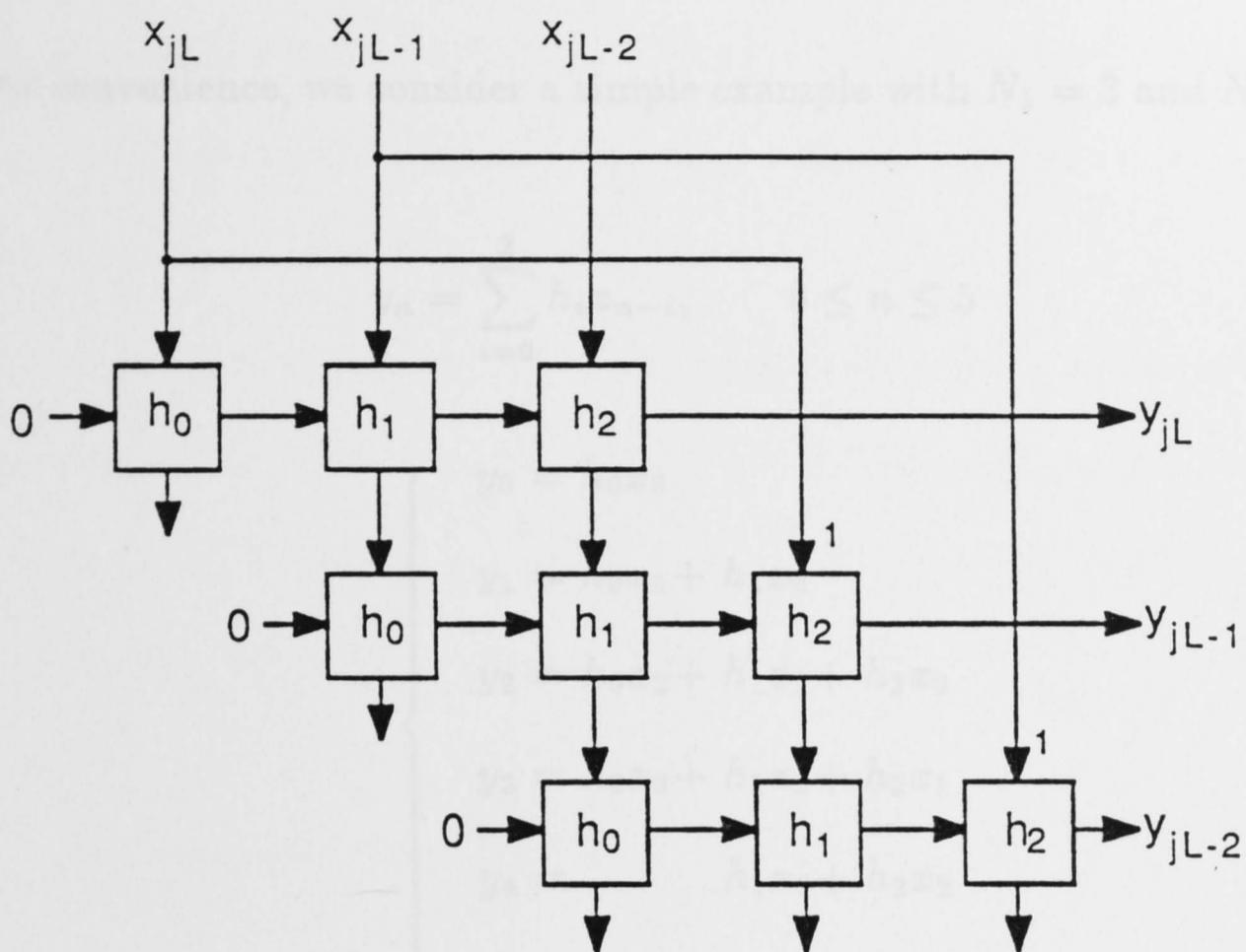
**Fig. 3.8.** The  $L \times N_1$  systolic array for solving linear convolution problems
