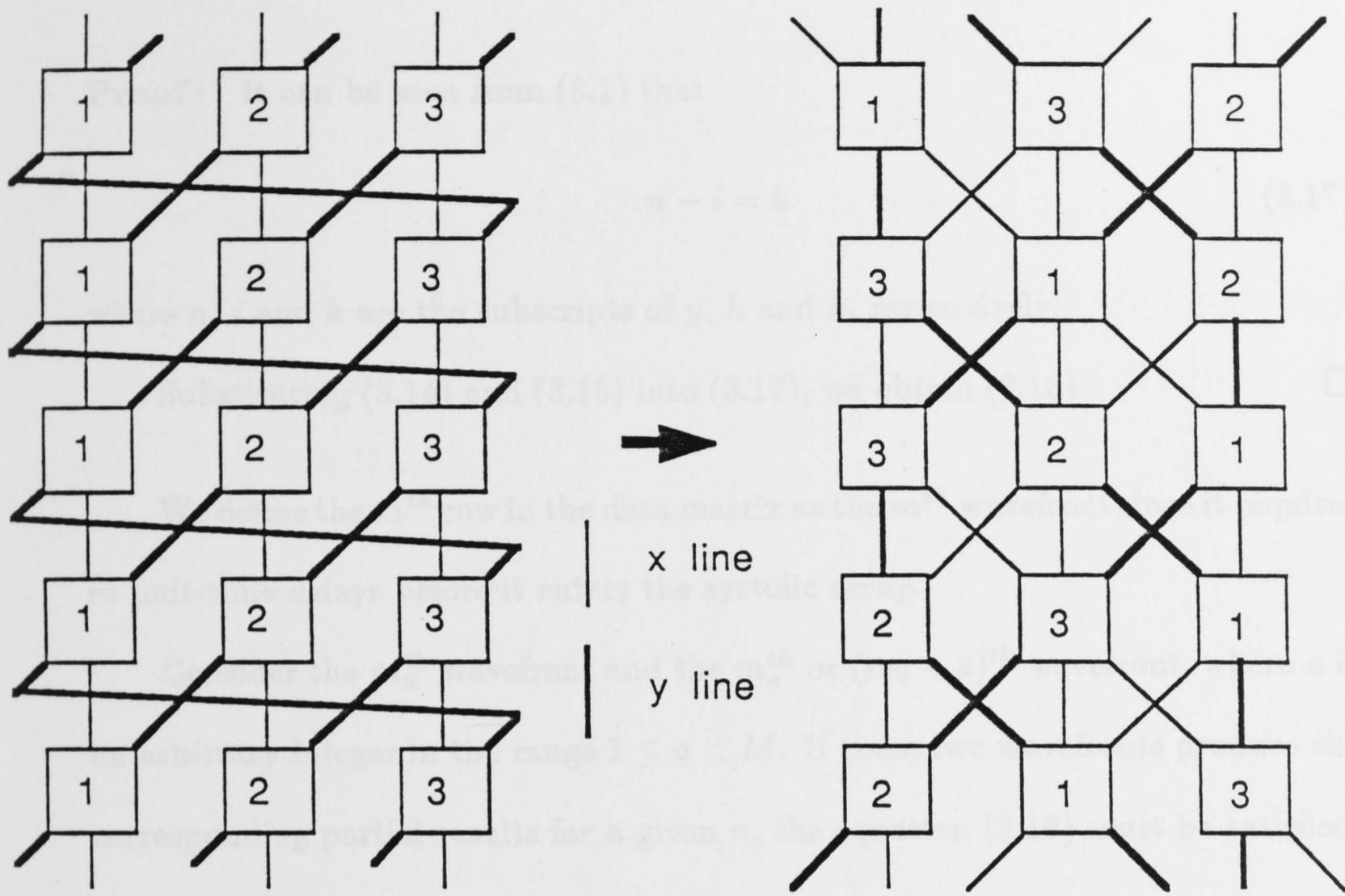
**Fig. 3.13.** Systolic layout of the 2-D systolic ring structure for solving linear convolution problems
