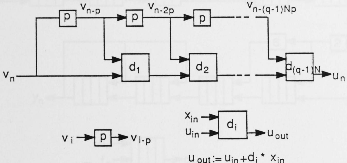
Fig. 5.2. The structure for computing (5.4)
