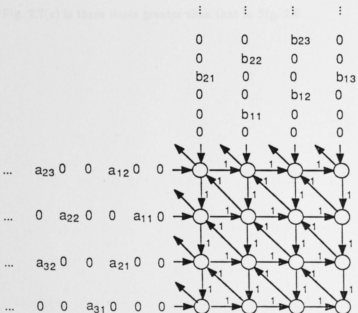
Fig. 2.6. Systolic array for multiplication of two band matrices in [24]
