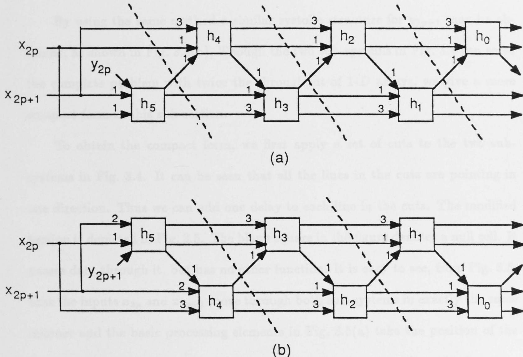
**Fig. 3.4.** 2-D systolic arrays (a) for computing  $y_{2p}$  and (b) for computing  $y_{2p+1}$
