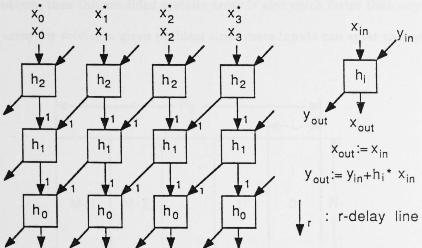
**Fig. 3.9.** An  $N_1 \times N_2$  systolic array for solving linear convolution problems
