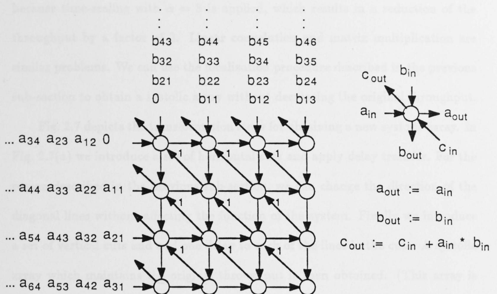
Fig. 2.5. SFG array for multiplication of two band matrices
