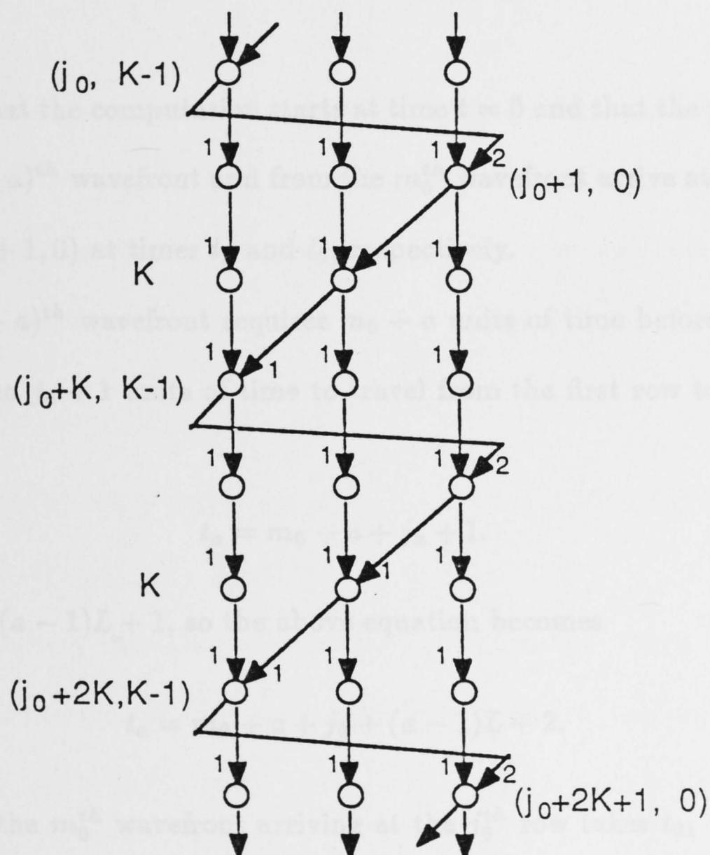
**Fig. 3.14.** The route for one output in the ring structure
