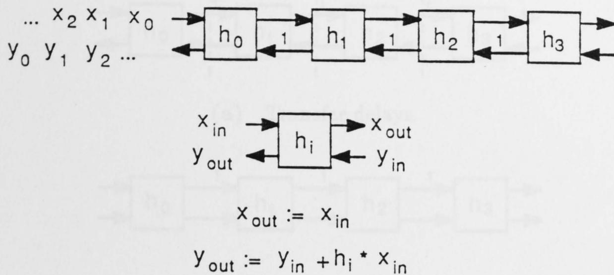
Fig. 2.2. SFG array for linear convolution
