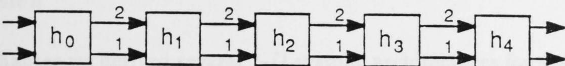
**Fig. 3.17.** A systolic ring structure with  $L = 1$
