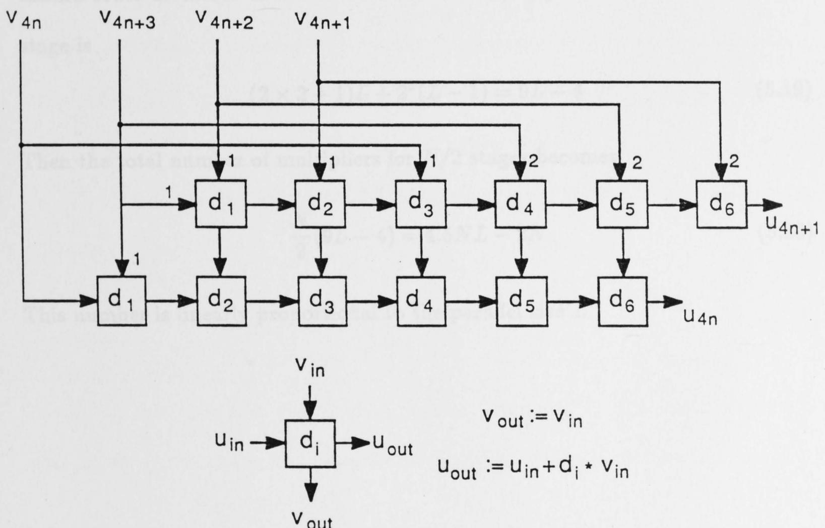
Fig. 5.8. The structure for computing  $u_{4n+l}$  for  $0 \leq l \leq 1$
