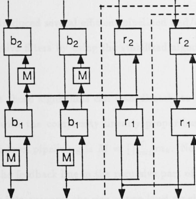
**Fig. 5.9.** The structure with  $M$  stages of second-level pipeline
