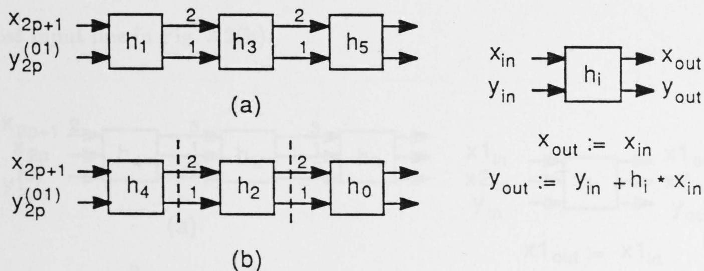
Fig. 3.2. Two equivalent systolic arrays for computing  $y_{2p}^{(01)}$  ( $N_1 = 6$ )
