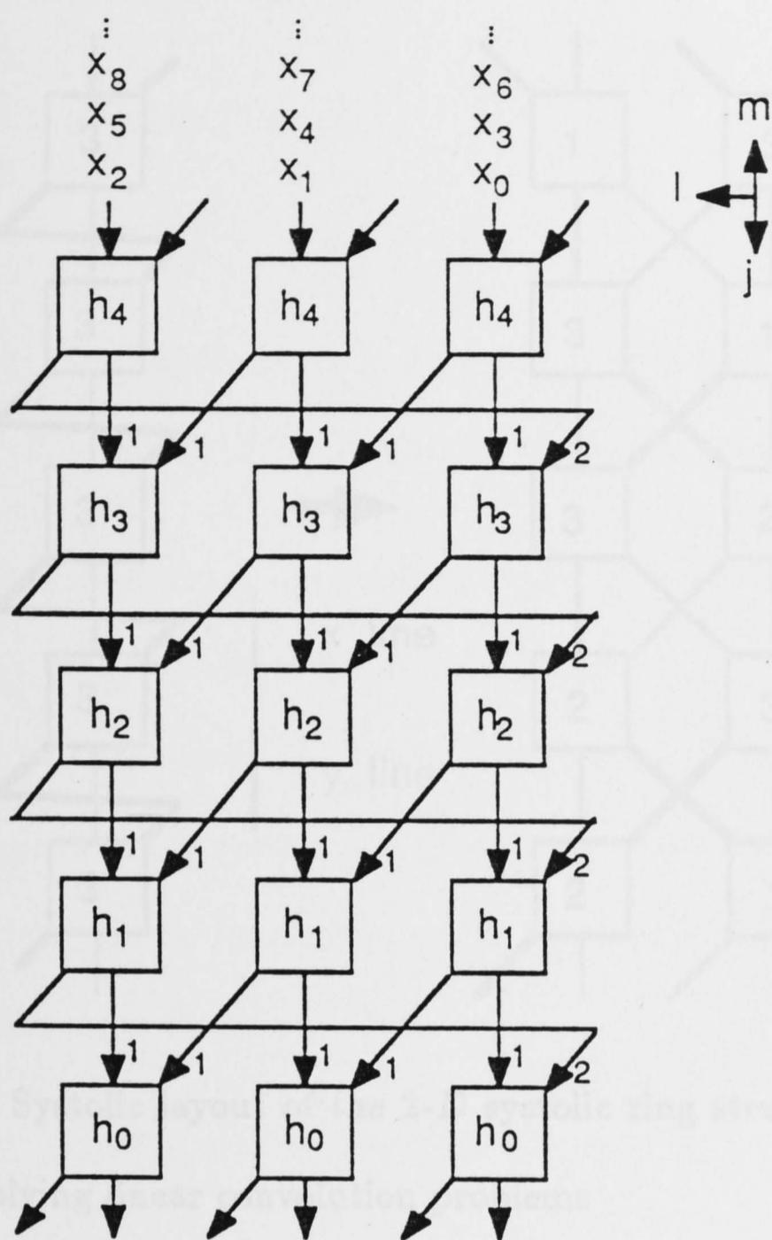
**Fig. 3.12.** An  $N_1 \times L$  ring structure for solving linear convolution problems
